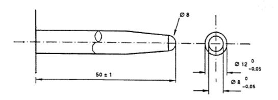
Discharge electrode: dimensions in mm
