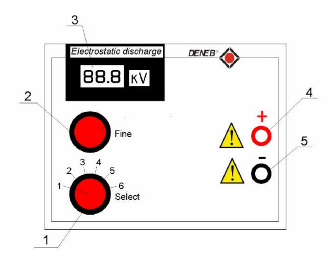
Through the selector 1 (SELECT) it is possible to choice the output voltage level and display it on the LCD 3.
